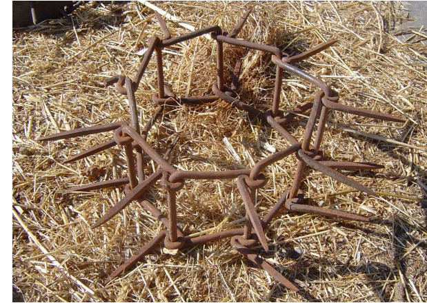
"Vreccale" or "Roccale": mesh example; usually the making of these protective metal collars was entrusted to the apprentices smiths http://commons.wikimedia.org/wiki/File:Roccale_1.jpg
